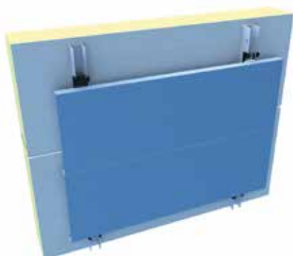
Hybrid FC panel on sandwich element: horizontal, parallel
