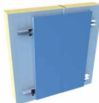
Hybrid FC panel on sandwich element: vertical, parallel
