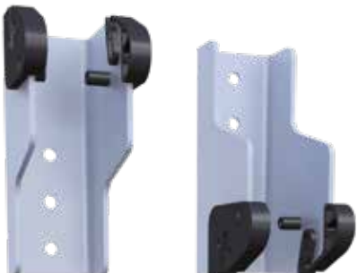
FC adapter for SE rail Length 94 mm, depth 53 mm without inlay, 3 holes, hole diameter: 5.2 mm
