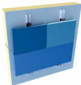
Hybrid FC panel on sandwich element: horizontal, offset
