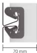
System depth with modular click rail SE
