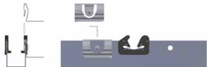
Number and arrangement of flashing support angles: approx. 1.5 units/m (arranged offset)
