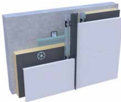
SE modular click rail on a horizontal substructure
