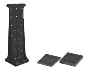
The new Kalzip Generation connecting clip for fastening Kalzip aluminium profiled sheets minimises thermal bridges, permitting a roof structure whose heat transfer rate is determined by the thermal insulation. The Kalzip Type E composite clip consists of a strong steel core enclosed in glass-fibre reinforced plastic.
