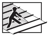
The protective film on the profiled sheets not only protects them during transport, but also while they are being zipped. It is important to make sure that this film is removed from the small seam prior to zipping.
